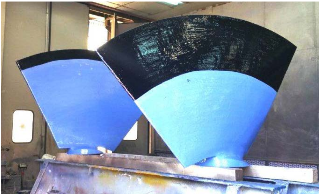
→ Kaplan turbine blades protected with Belzona I3II, I34I and 2I4I
